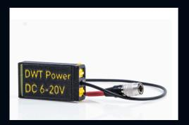
Hirose power supply for Sony DWX for use with DWT-B01, DWT-B30, DWT-P01 · 4-pin Hirose connector with 40cm cable · Input 6V-20V
