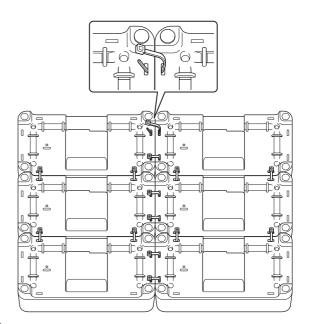
4 Connect the cables, insert the cable ties through the holders on the bottoms of the units, and secure them while grouping the cables.
