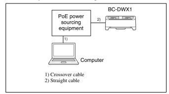
• When multiple units and other devices are connected
