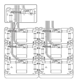
The holes at the bottom of the units that are not being used for connections can be used to secure the units to the tray or drawer of a commercially available 19-inch rack, for example.
