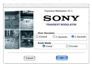
The menu allows the selection of overload indication duration between 'permanent until reset', 5 seconds or 2 second auto-reset modes. The GUI knob mode can also be selected for control operation in linear or circular modes.
